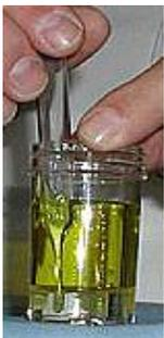
Place the tip of the test ampoule down into one of the slots in the bottom of the filled Sample/ Snapping Cup.
