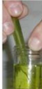
Pull back on the top to break the ampoule tip. Keeping the ampoule in the water. The ampoule will automatically fill with the sample water.
